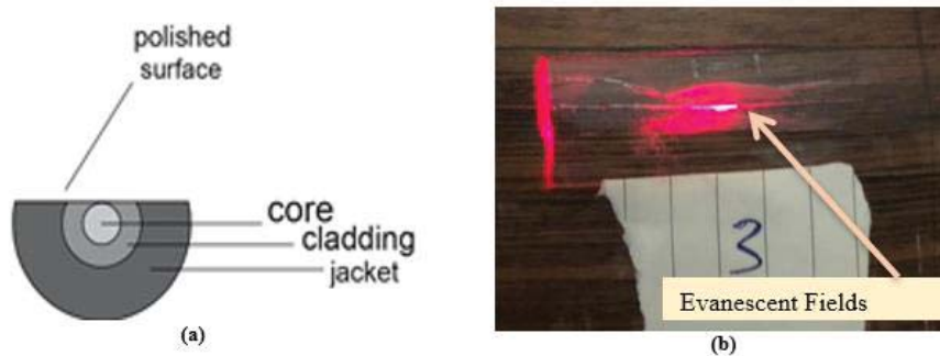
FIGURE 3. (a) Side view of D-Shaped Fiber (b) Propagation evanescent field
