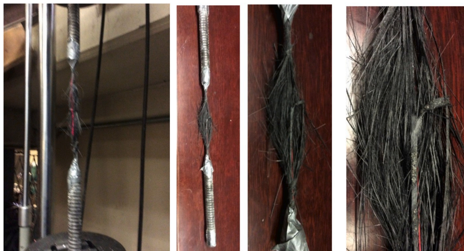
Fig. 2. Failure modes for No.6 CFRP bar.
