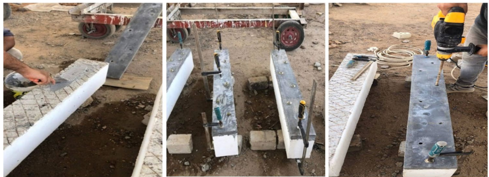
Fig. 4 Fixing Precast SIFCON layer with beam by epoxy, bolts, and applied weight
