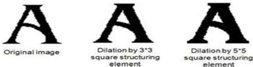
Figure (2.12): Dilation process [8]
