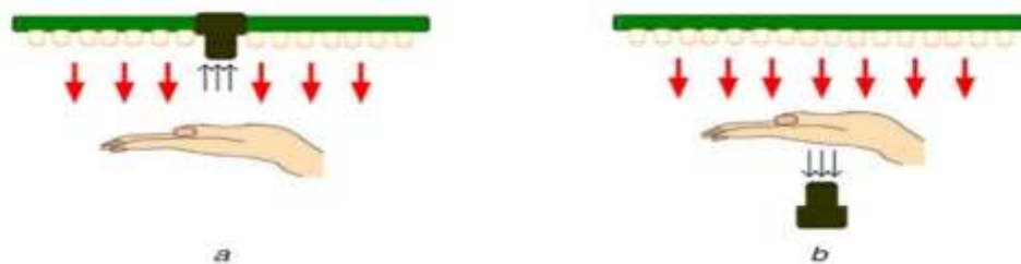
Figure (2.5): capturing the image of palm vein methods (a) Method of refraction (b) Method of transmission [2]
