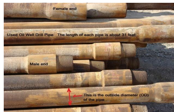
Figure 3. The oil drilling pipe body
