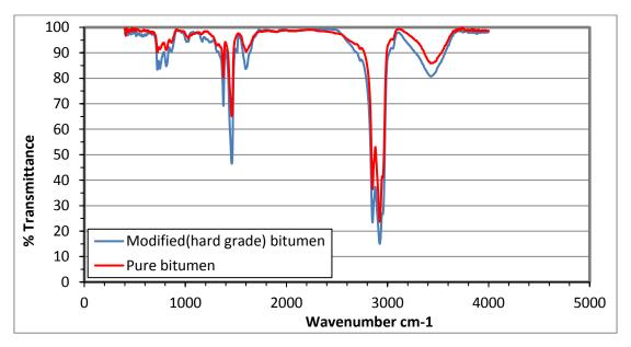
Figure 10. FTIR test results for pure and hard grade bitumen
