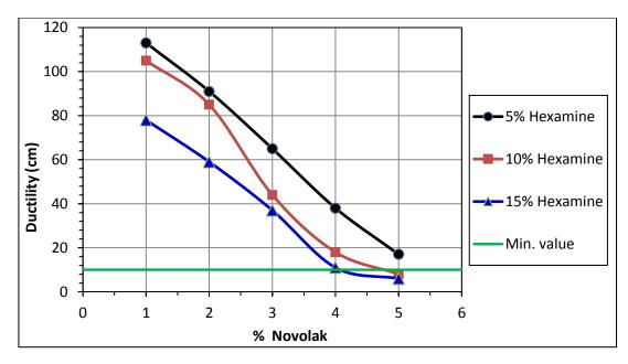
Figure 9. Ductility of bitumen has different ratios of Novolac and Hexamine [6].
