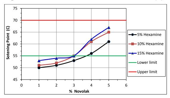
Figure 8. Softening point of bitumen has different ratios of Novolac and Hexamine [22].
