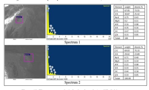
Figure 12. Elementary analysis for hard grade (modified) bitumen
