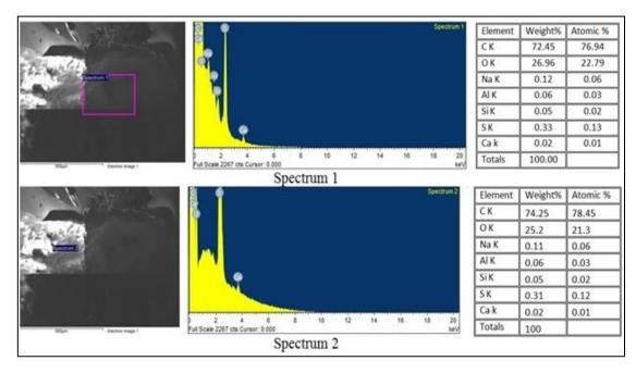
Figure 11. Elementary analysis for conventional 40-50 (unmodified) bitumen
