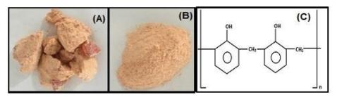
Figure 1.Novolac (Phenol formaldehyde solid resin) :( A) Novolac particles, (B) Grinded Novolac, (C) Structure of Novolac [20].
