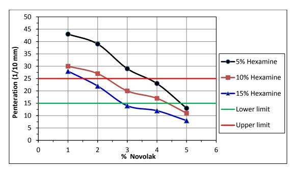
Figure 7. Penetration of bitumen has different ratios of Novolac and Hexamine [22].
