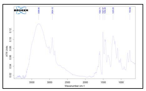
Figure 5. FTIR test results of Novolac
