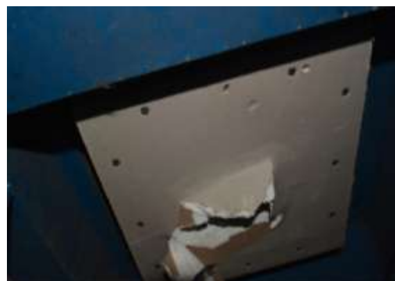
(b) Assemblies fastened with 3 bolts
