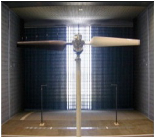
Fig. 1. The NREL Phase VI rotor geometry [25].
