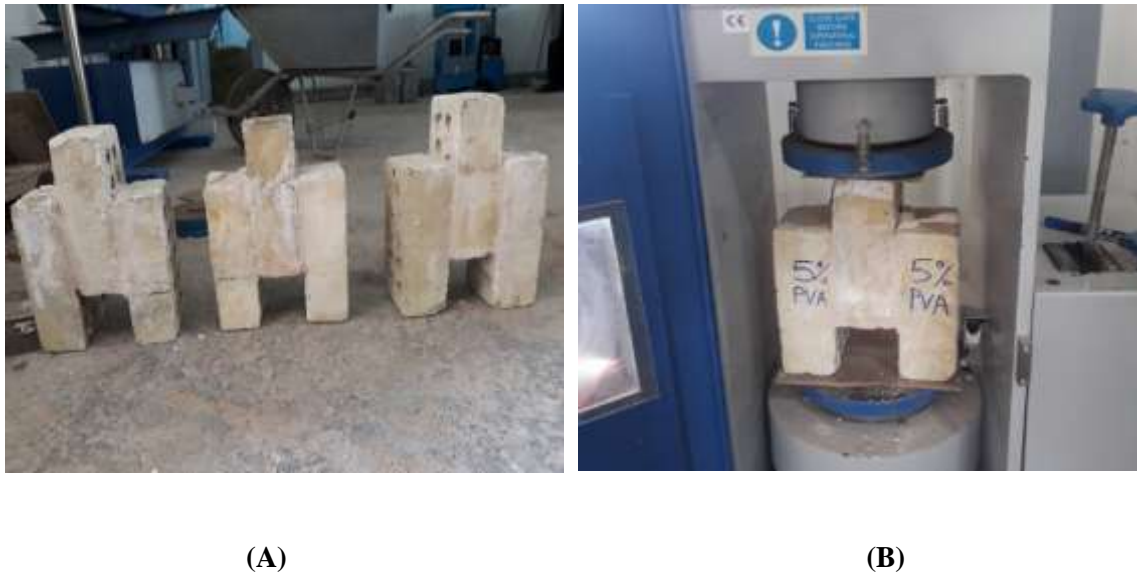
Figure 1 (A) Bricks arrangement in the masonry unit, (B) Shear bond strength test
