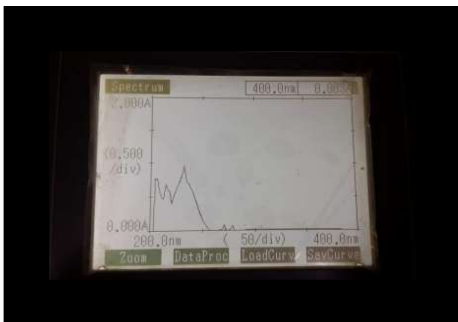
Figure 1 , \lambda_{\max} of metformin that obtained
