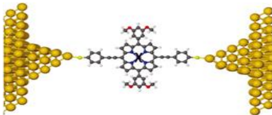
Figure 3.4. An example of an optimized junction configuration. To reduce the computational cost, we replace the electrically-inert alkyl group ( -C_8H_{17} ) with a methyl group ( -CH_3 ).[2]
