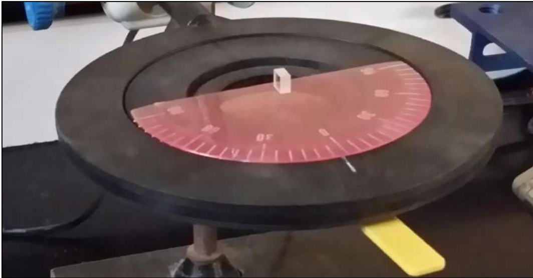
Figure (3-9) crystal thickness tilts using bevel protractor.
