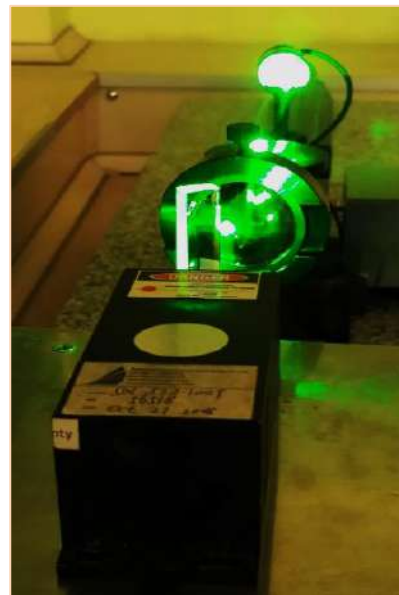
Figure (3-6) the set – up of Optical Limiting for (KTiOPO 3 )
