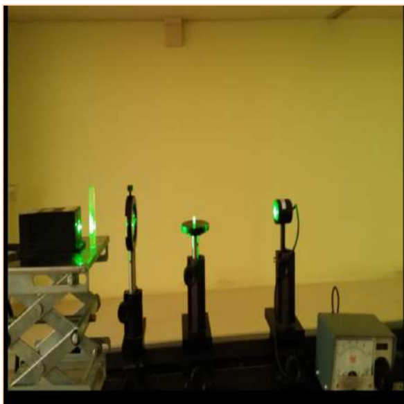
Figure (3-6) the set – up of Optical Limiting for (KTiOPO 3 )
