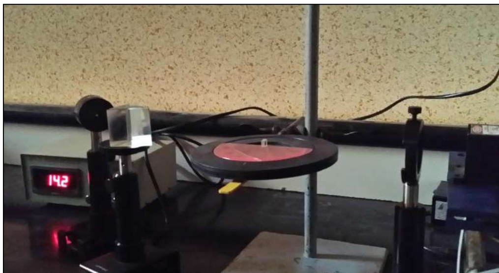
Figure (3-8 ) the set-up of SHG measurements at wavelength 1064nm
