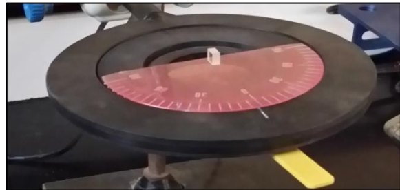
Figure (5) crystal thickness- tilts using bevel protractor.
