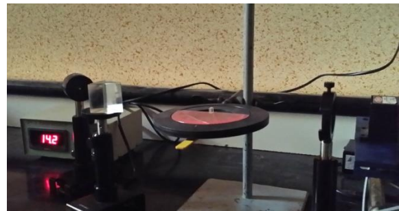
Figure (4) the set-up of SHG measurements at wavelength 1064nm
