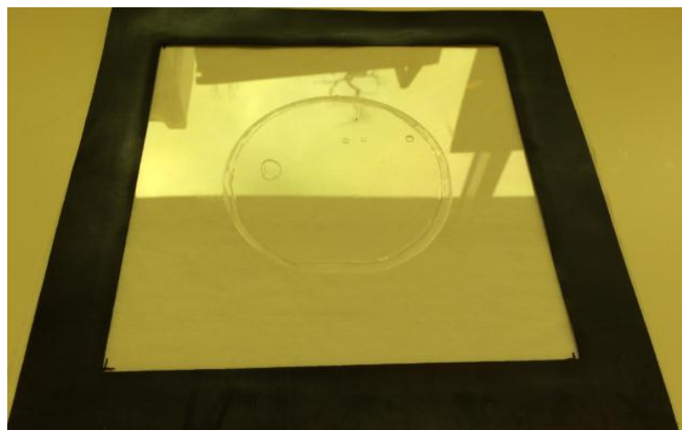
Figure 16 displays the rubber stamp on a glass sheet with a black rubber ring
