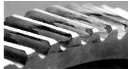
Fig.1. Micropitting pattern on a helical wheel. (Erichello, 2012).
