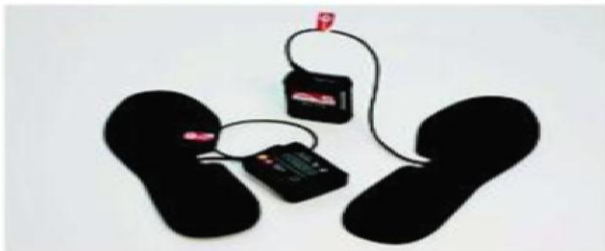
● Foot sensors with weight bearing insoles
