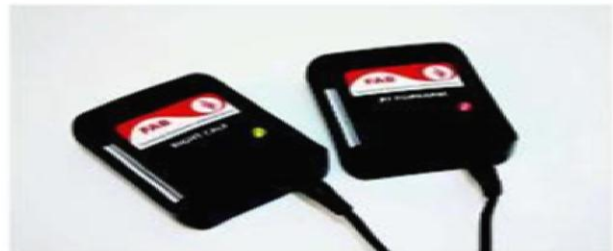
● LEDs display sensor battery status
