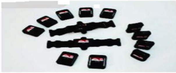
● FAB wireless 3D motion sensors
