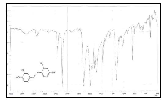
Figure (2) The FTIR Spectra of AZO2
