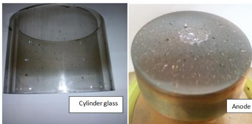
Figure 5 shows pictures from the cathode and the anode and the cylinder glass after each arcdischarge
