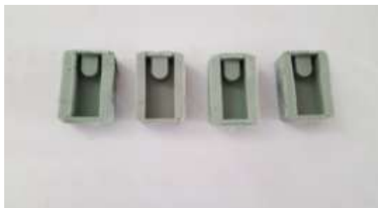
Fig (3) A: Polysiloxane U-shaped mold
