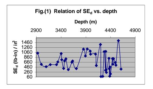
We notice that each point on the graph represent bit performance regardless the trip time, rig cost, and other parameters that effects the cost per foot (CPF). We will show later how the best bit performance carried lowest values of  $SE_d$  values.
