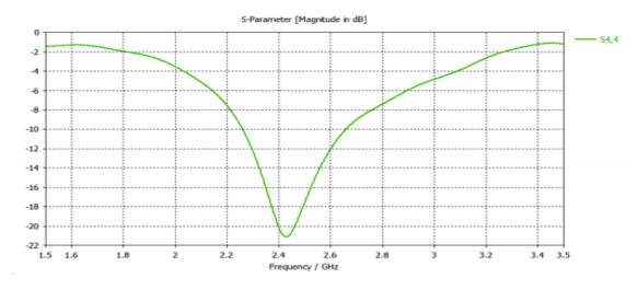
Fig.4 Return loss, S33 vs. Frequency
