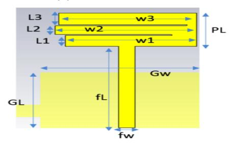
Fig.1 View of the proposed LTE patch with the ground transparency
