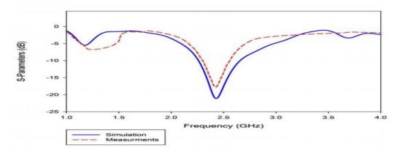
Fig.10 Simulation and measurement Antenna Loss for port 4
