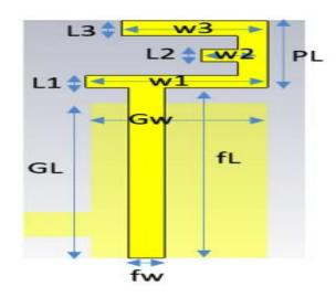
Fig.2 View of the proposed WIFI patch with the ground transparency
