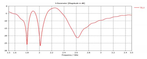
Fig.3 Return loss, S11 vs. Frequency
