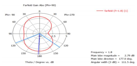
Fig.6 polar far field view at 1.8 GHz, phi=90
