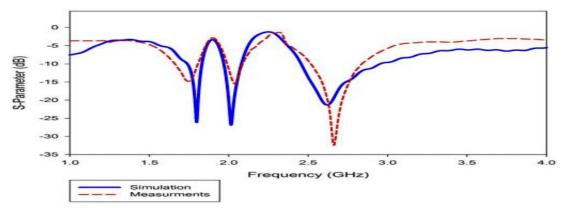
Fig.9 Simulation and measurement Antenna Loss for port 1
