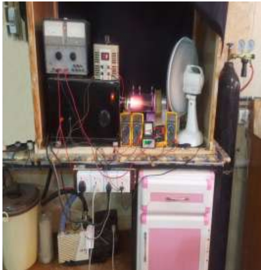
Figure 1 represents discharge unloading system dc Figure ( 1) illustrates the scheme for electric circuit used to measure the voltage collapse of gases
