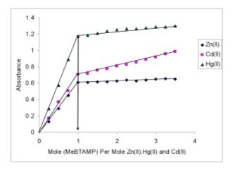
Fig.(7):- Mole ratio method (M:L) (MeBTAHP) -metal chelates Zn(π),Cd(π) and Hg(II).
