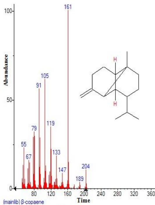
**Fig. 10: Structure of  $\beta$ -copaene with RT: 10.606 present in *Cassia fistula***
