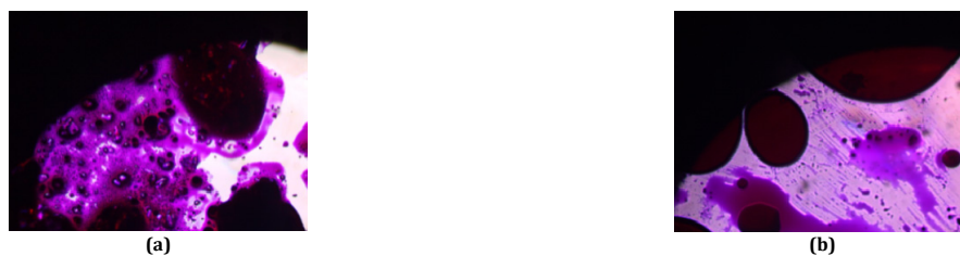
Figure 6. Images of polarized optical microscope for compound 5, (a) Crystal phase (30 °C heating) (b) Liquid phase (100 °C heating).
