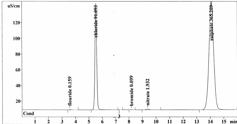
Figure 1. Chromatogram of common anions in raw water sample for East Tigris Plant.
