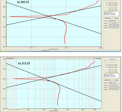
Figure (3) : The anodic and cathodic polarization curves in 0.1 mol dm<sup>-3</sup> aerated hydrochloric acid solution in the presence of 7.87×10<sup>-5</sup> mol dm<sup>-3</sup> of inhibitor I at 293.15 K , 303.15K and 313.15K , respectively .
