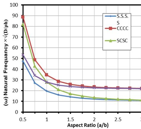
**Figure (6):** Finite difference natural frequencies of curved plate with different boundary conditions and aspect ratios
