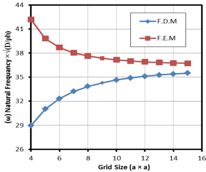
**Figure(4):** Finite difference versus Finite Element Results for a Clamped supported curved plate
