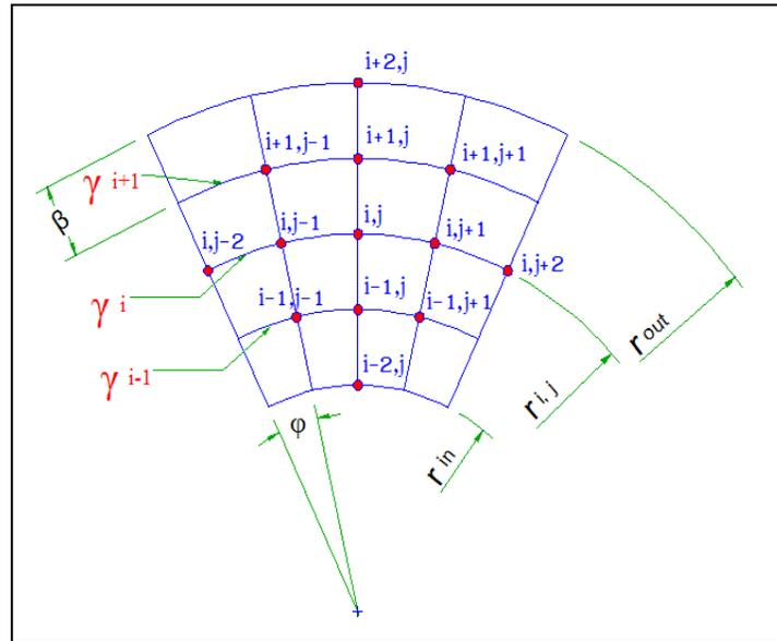
**Figure (1):** Geometry of the curved plate and node distribution
