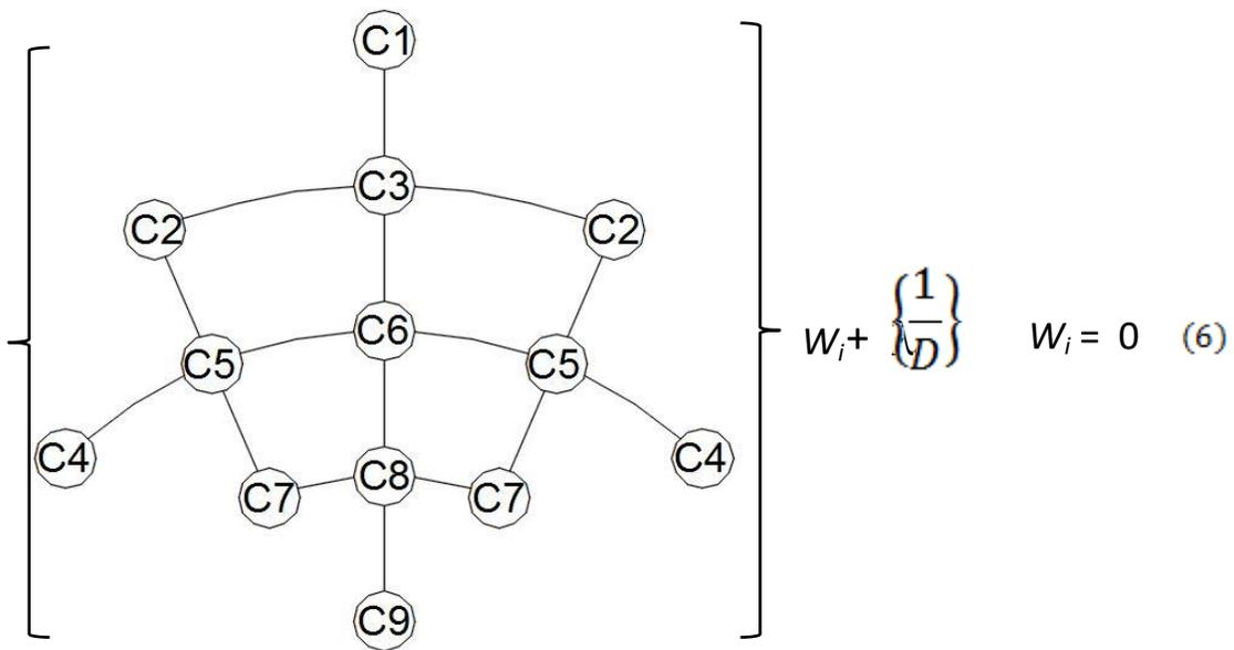
**Figure (2):** Finite difference scheme of curved plate differential equation
