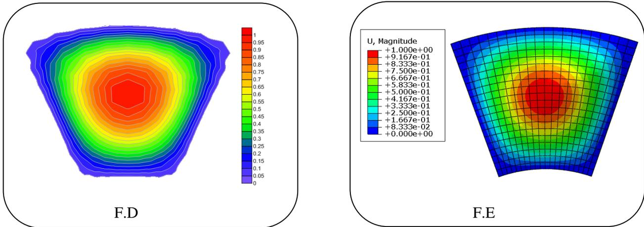
**Figure (5):** Deflection values for first mode of SSSS plate for finite difference and finite element
