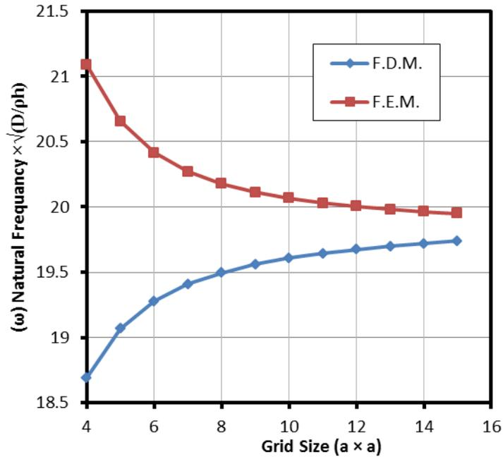
**Figure(3):** Finite difference versus Finite Element Results for a simply supported curved plate
