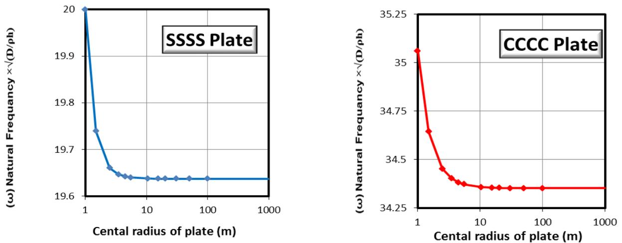
**Figure (7):** Finite difference natural frequencies of curved plate with different boundary conditions and different radii
