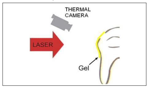
Fig (3) Experimental set-up for measuring get temperature dynamtics during laser –assisted tooth whitening [2].
