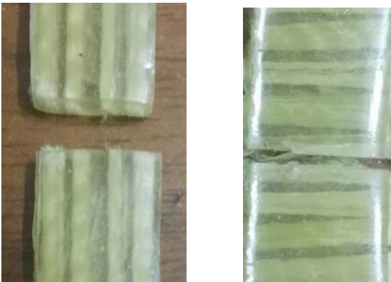
Figure 7 : The fracture direction Vs. fiber direction.
