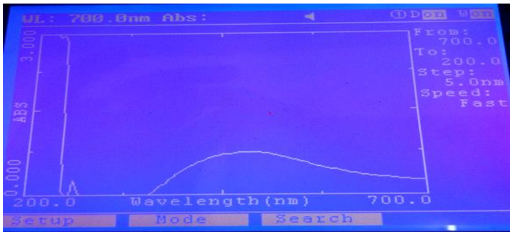
Figure(3.2): A Peak(430) of silver nanoparticles synthesized by Agaricus bisporus after (24, 48 and 72 hours) by UV-visible spectroscopy .
